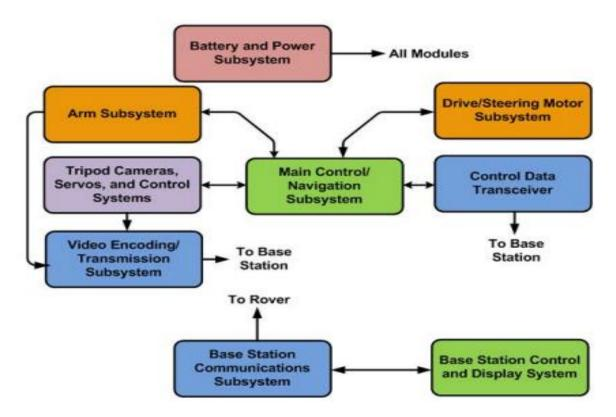
• **POWER SYSTEM:** Power system is used for providing the necessary electricity to run the rover's systems. The batteries we are using is of [12V 10(amp)] and [9V]
